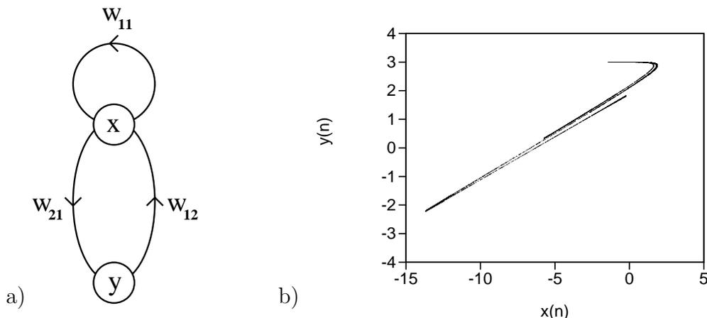
Figure 1: a) The chaotic module consisting of a self- inhibitory neuron with activity  $x_n$ , and an excitatory neuron with acitivity  $y_n$  at time step  $n$ . b) The chaotic attractor of this module for parameters as in equation (2).
