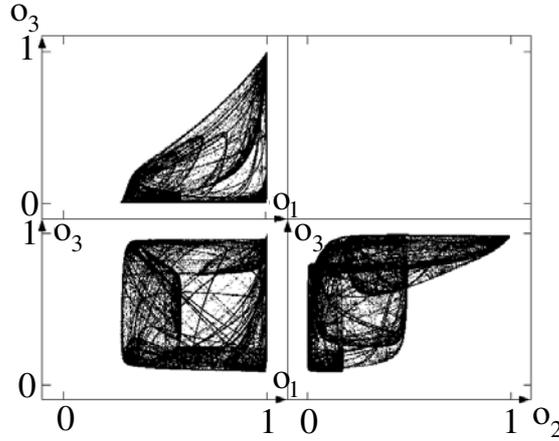
**Figure 18.** 3-ring 4.3: three projections of a chaotic attractor in the  $(o_1, o_2, o_3)$ -output space for parameter values  $-w_{21} = -w_{31} = w_{23} = w_{12} = w_{32} = w_{13} = 8, \theta_1 = -1.75, \theta_2 = 0, \theta_3 = 5.5$ .
