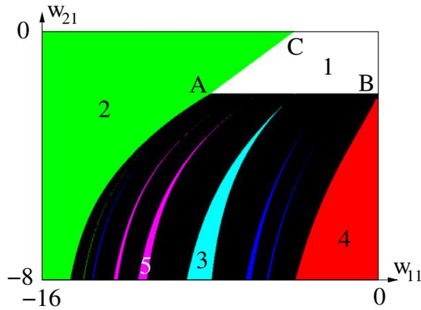
**Figure 9.** 3-chain 4.1: iso-periodic plot in the  $(w_{11}, w_{21})$ -parameter subspace for which the origin  $a^* = 0$  is always a fixed point (see the text for parameters). Numbers  $r$  refer to the existence of period- $r$  attractors.
