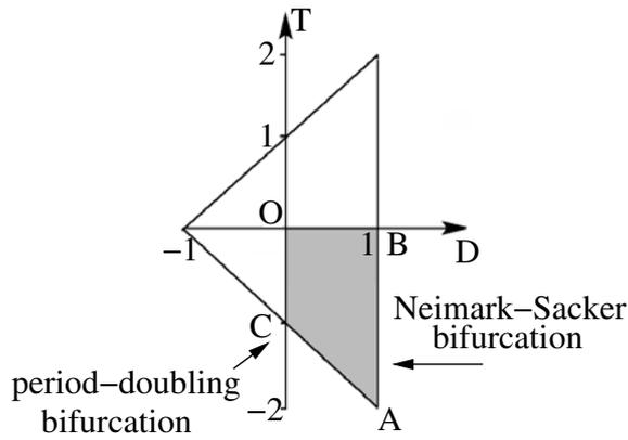
**Figure 2.** The stability domain for a fixed point in terms of trace  $T$  and determinant  $\mathcal{D}$  of the linearization  $Df_\rho$ ; the shaded domain corresponds to recurrent coupling of a self-inhibitory with an excitatory neuron.
