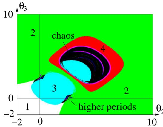
**Figure 10.** 3-chain 4.1: iso-periodic plot for  $(\theta_2, \theta_3)$ -parameter subspace for  $w_{12} = w_{13} = 4$ ,  $w_{21} = w_{31} = -6$ ,  $w_{11} = -16$ ,  $\theta_1 = -3.4$  fixed. Numbers  $r$  refer to the existence of period- $r$  attractors.
