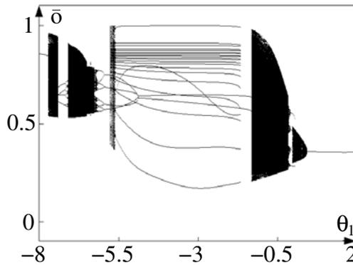
**Figure 17.** 3-ring 4.3: a bifurcation diagram for  $\theta_1$  with parameters  $\theta_2 = 1, \theta_3 = 5.5, -w_{21} = -w_{31} = w_{23} = w_{12} = w_{32} = w_{13} = 8$  fixed. Plotted is the averaged output  $\bar{o}$  of the module.
