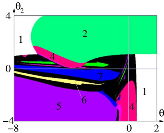
**Figure 16.** 3-ring 4.3: iso-periodic plot in the  $(\theta_1, \theta_2)$ -parameter subspace with fixed parameters  $-w_{21} = -w_{31} = w_{23} = w_{12} = w_{32} = w_{13} = 8, \theta_3 = 5.5$ . Numbers  $r$  refer to the existence of period- $r$  attractors.
