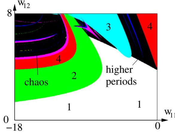
**Figure 1.** Chaotic 2-module: iso-periodic plot in the  $(w_{11}, w_{12})$ -subspace for fixed parameters  $w_{21} = -6, \theta_1 = -3, \theta_2 = 4$ . Numbers  $r$  refer to the existence of period- $r$  attractors.
