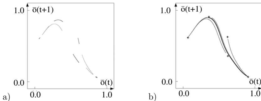
**Figure 7.** Chaotic 2-module: for parameters  $\theta_1 = -1.75$ ,  $w_{11} = -16$ ,  $w_{12} = 6$ ,  $w_{21} = -6$  one observes (a) a 2-cyclic chaotic attractor (grey) co-existing with a 5-cyclic one (black) for  $\theta_2 = 2.78$ , and (b) a chaotic attractor co-existing with a period-5 attractor (stars) for  $\theta_2 = 3.25$ , displayed in terms of the first return map of the averaged output  $\bar{o}$ .
