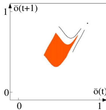
**Figure 14.** 3-chain 4.2: first return map of two chaotic attractors (grey area and the two lines) co-existing with one fixed point attractor for parameter values  $-w_{21} = w_{23} = w_{12} = w_{32} = 8$ ,  $\theta_1 = -3$ ,  $\theta_2 = 5.65$ ,  $\theta_3 = -7$ . Plotted is the averaged output  $\bar{o}$  of the module.
