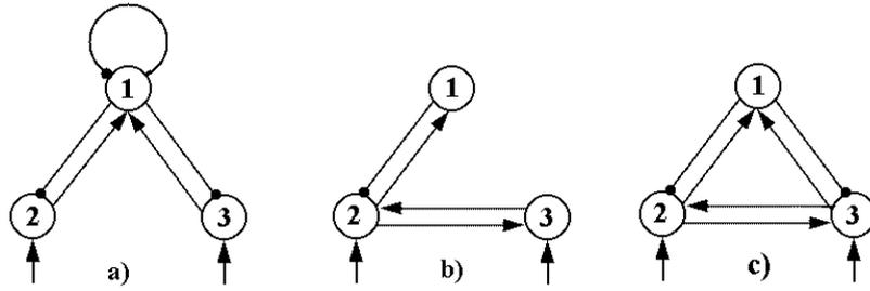
**Figure 8.** Three examples of three-neuron modules, all with one inhibitory neuron. Arrows denote excitatory, dots inhibitory connections.
