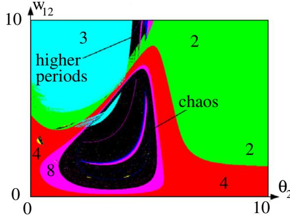
**Figure 11.** 3-chain 4.1: iso-periodic plot for  $(\theta_2, w_{21})$ -parameters with  $\theta_1 = -2$ ,  $\theta_3 = 3.4$ ,  $w_{11} = -16$ ,  $w_{21} = w_{31} = -6$ ,  $w_{13} = 4$  fixed. Numbers  $r$  refer to the existence of period- $r$  attractors.
