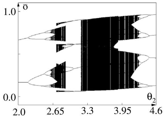
**Figure 6.** Chaotic 2-module: bifurcation sequence for  $\theta_2$  of the chaotic 2-module with  $\theta_1 = -1.74$ ,  $w_{11} = -16$ ,  $w_{12} = 6$ ,  $w_{21} = -6$ , indicating co-existing chaotic attractors around  $\theta_2 = 2.75$ . Plotted is the averaged output  $\bar{o}$  of the module.
