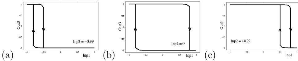
Figure 4: *Hysteresis domain of  $Inp1$  for output neuron  $Out3$  of the network (fig. 1(a)) with  $Inp2$  fixed.*
